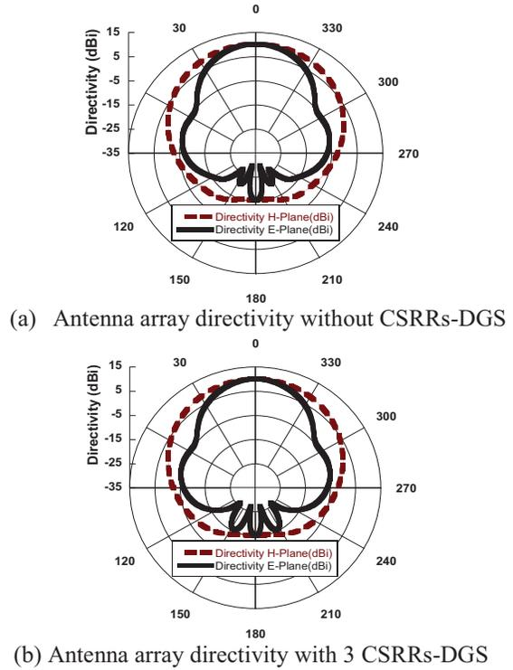
Fig. 3. Optimized antenna array radiation pattern results with and without 3 CSRRs-DGS at 9.22 GHz.
