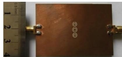
(b) Photograph of the fabricated antenna array (Bottom view)
