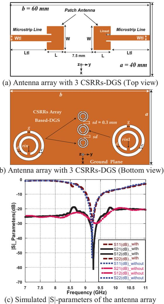
Fig. 2. Antenna array configurations and simulated  $|S|$ -parameters with and without CSRRs-DGS.
