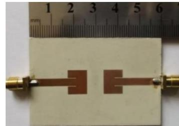
(a) Photograph of the fabricated antenna array (Top view)
