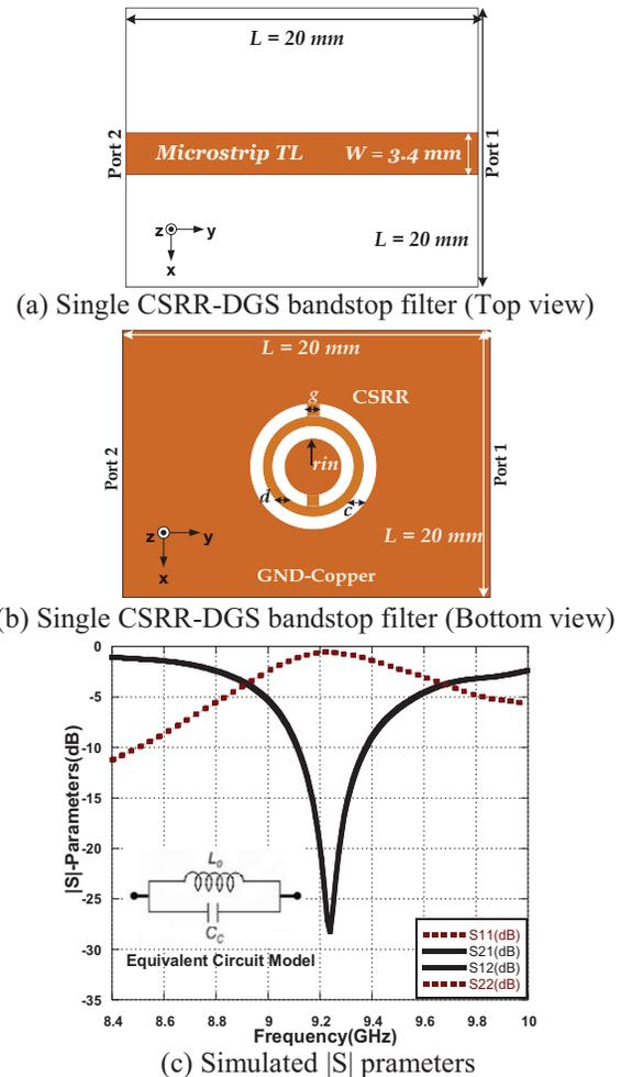
Fig. 1. Schematic of the optimized CSRR-DGS bandstop filter and  $|S|$ -parameters results.
