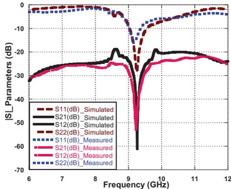
(d) Measured and simulated  $|S|$  parameters of the proposed array with 3 CSRRs-DGS
