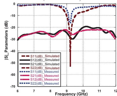
(c) Measured and simulated  $|S|$  parameters of the conventional array without CSRRs-DGS
