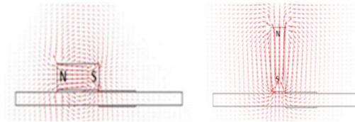
Fig. 9. Direction of magnetic flux density for magnet in horizontal and vertical position.
