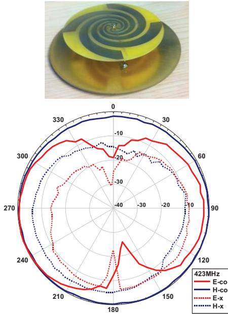
Fig. 1. Multi-element low profile spiral antenna prototype and its measured radiation pattern in principal E-plane and H-plane co-polarization and cross-polarization.
