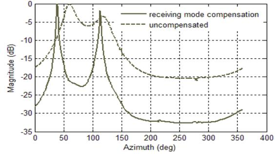
Fig. 7. MUSIC spatial spectrum for two incident signals with azimuth angles of 40 and 110 degrees, six-element low profile spiral array.
