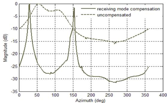
Fig. 6. MUSIC spatial spectrum for two incident signals with azimuth angles of 30 and 150 degrees, four-element low profile spiral array.
