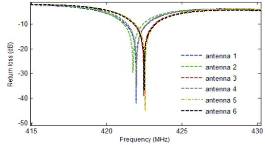
Fig. 3. Measured return losses of low profile spiral antennas
