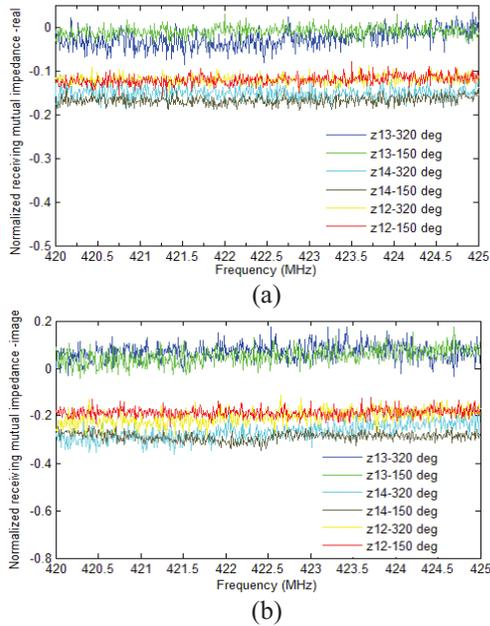
Fig. 4. Normalized mutual impedance for AOA = 150 and 320 degrees over the frequency band: (a) real part and (b) imaginary part.
