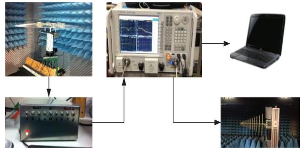
Fig. 5. Data acquisition setup for the AOA estimation experiment.
