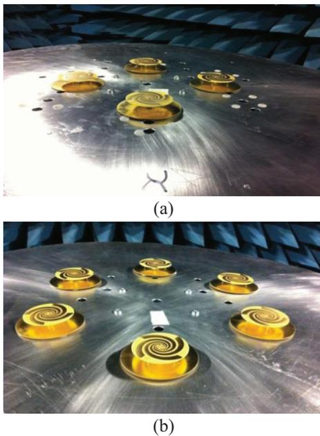
Fig. 2. Antenna array geometries used for data acquisition.
