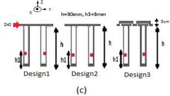
Fig. 1. The employed designs: (a) top view, (b) slot dimension and excitation probe length, and (c) side view (L<sub>p</sub> is length of excitation probe, h is height of backed cavity and h<sub>1</sub> is place of probe from the back of structure).
