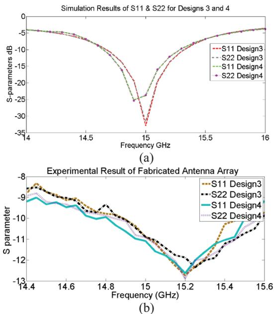
Fig. 11. (a) Simulated and (b) measured  $S_{11}$  and  $S_{22}$  for design 3 and 4.
