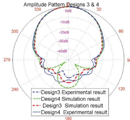
Fig. 13. Amplitude pattern of simulation and experimental results.
