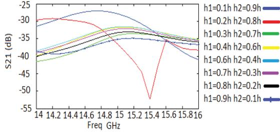
Fig. 6. Simulation result of mutual coupling for different capacitive and inductive parts.
