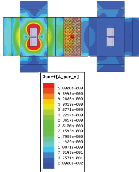
Fig. 8. EM-EBG effect on current distribution for design 4.
