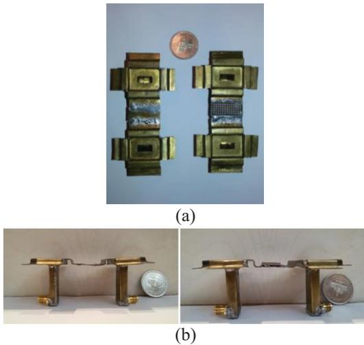
Fig. 9. Fabricated cavity backed slot antenna non-planar array: (a) top view and (b) side view (left) design 3, (right) design 4.
