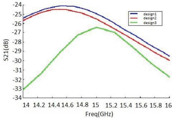
Fig. 4. Mutual coupling extracted by HFSS simulator for the three designs.
