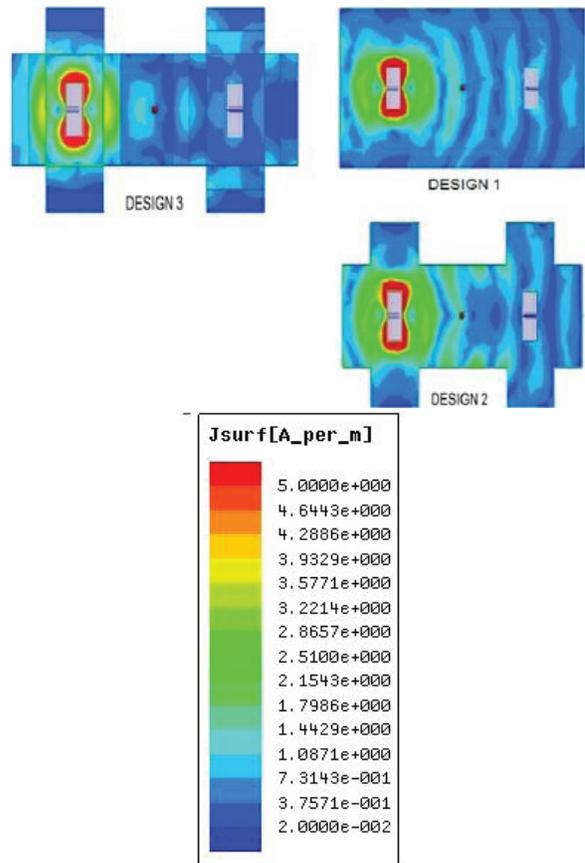
Fig. 2. Current distribution on the three designs.
