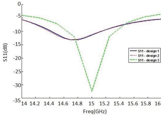
Fig. 3. Reflection coefficient,  $S_{11}$  for designs 1, 2 and 3.
