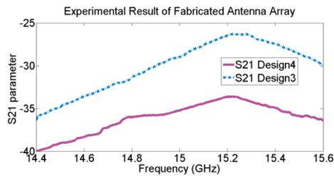
Fig. 10. Mutual coupling improvement by applying tuned EM-EBG.
