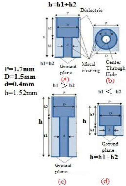
Fig. 5. An EM-EBG cell is composed by two metalized holes (vias) with two different diameters. Diameter of the top hole is ( $D$ ) and the other hole is ( $d$ ). (a) Side view of normal EM-EBG ( $h_1=h_2=h/2$ ), (b) top view, and (c) tuned EM-EBG, the first case ( $h_1 < h_2$ ) tuned EM-EBG, the second case ( $h_1 > h_2$ ).
