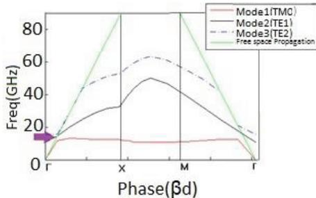
Fig. 7. Dispersion diagram of the tuned EM-EBG cell.
