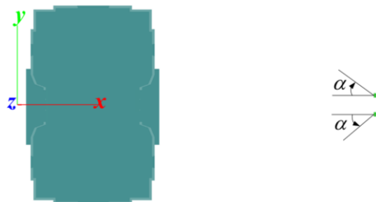
Fig. 10. Main-lobe directions of base-station antennas in the xoy plane.
