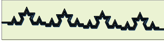
Fig. 4. A second-order Koch-shaped microstrip filter.
