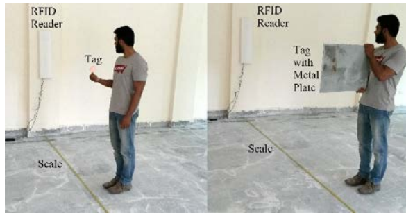
Fig. 12. Measurement setup for readrange.
