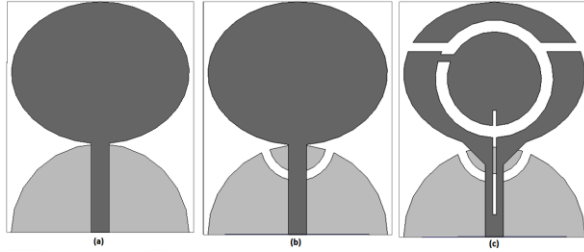
Fig. 3. (a) The ordinary elliptical patch and half circular shape ground plane. (b) The antenna with slotted ground plane. (c) Proposed antenna with defected ground plane and slotted patch.
