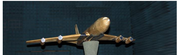
Fig. 1. Scale model setup in the compact range at the University of Pretoria, South Africa.
