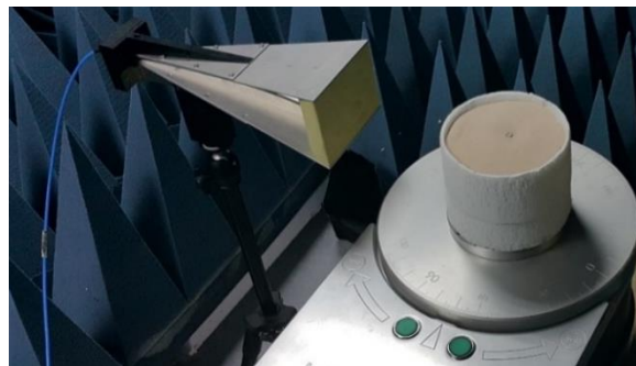
Fig. 5. Screw in sand filled foam container on the turntable.
