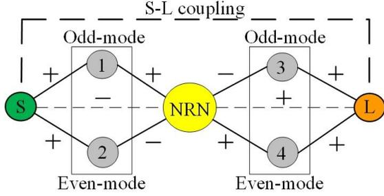
Fig.3. Coupling scheme of the proposed LTCC BPF.
