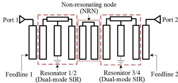
Fig. 1. Planar configuration sketch of the proposed BPF.
