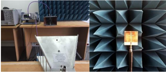
Fig. 9. Measurement setup for maximum far field gain.
