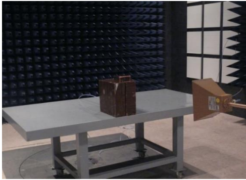
Fig. 6. SE measurement setup in EMC chamber.
