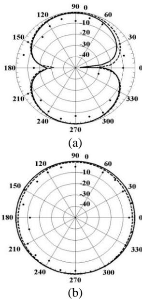
Fig. 7. Radiation patterns: (a) E-plane and (b) H-plane of the circular printed monopole antenna shown in Fig. 3 at 3 GHz (theory (—), simulation using HFSS (---), and measured (.) [4]).
