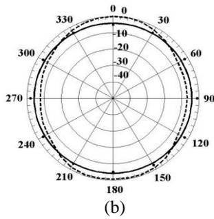
Fig. 5. Radiation patterns: (a) E-plane and (b) H-plane of the rectangular printed monopole antenna shown in Fig. 2 at 5.2 GHz (theory (—), simulation using HFSS (---), and measured (.) [3]).
