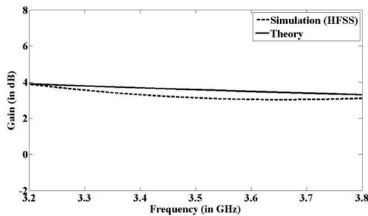
Fig. 6. Gain of rectangular printed monopole antenna on dielectric substrate ( $\epsilon_r = 4.3, \tan\delta = 0.02$ ) of thickness  $h=1.52$  mm.
