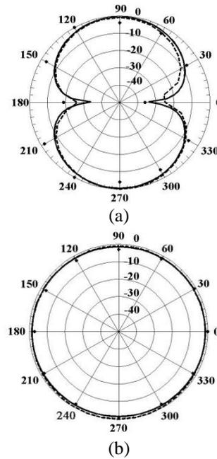
Fig. 4. Radiation patterns: (a) E-plane and (b) H-plane of the rectangular printed monopole antenna shown in Fig. 2 at 2.45 GHz (theory (—), simulation using HFSS (---), and measured (.) [3]).
