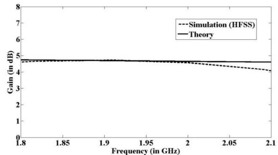
Fig. 9. Gain of circular printed monopole antenna on dielectric substrate ( $\epsilon_r = 4.7, \tan\delta = 0.02$ ) of thickness  $h=1.5$  mm.
