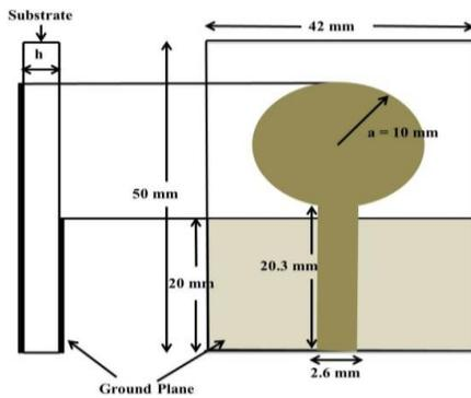
Fig. 3. Geometry of circular printed monopole antenna on dielectric substrate ( $\epsilon_r = 4.7, \tan\delta = 0.02$ ) of thickness  $h=1.5$  mm in [4].
