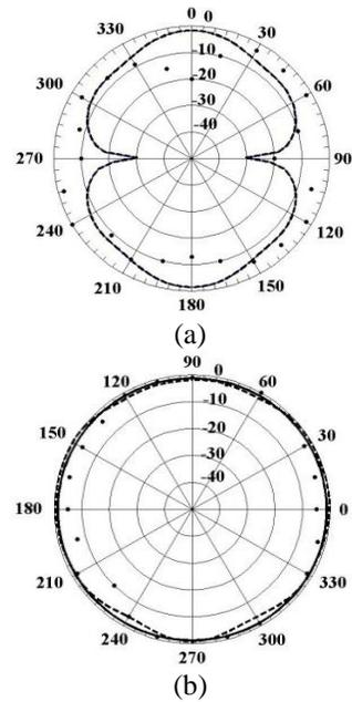
Fig. 8. Radiation patterns: (a) E-plane and (b) H-plane of the circular printed monopole antenna shown in Fig. 3 at 6.5 GHz (theory (—), simulation using HFSS (---), and measured (.) [4]).
