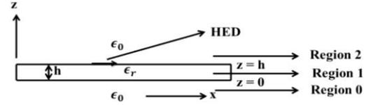
Fig. 1. Geometry of an HED along x-axis on the interface of dielectric and free space.
