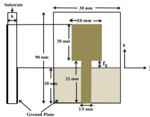
Fig. 2. Geometry of rectangular printed monopole antenna on dielectric substrate ( $\epsilon_r = 4.3, \tan \delta = 0.02$ ) of thickness  $h=1.52$  mm in [3].
