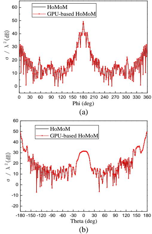
Fig. 11. 2D RCS of the airplane: (a)  $xoy$  plane and (b)  $xoz$  plane.
