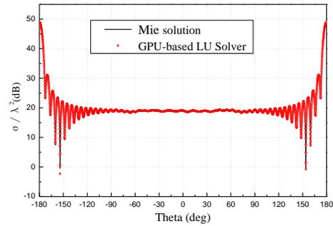
Fig. 7. RCS results in  $xoz$  plane from the PEC sphere with radius of  $10\lambda$ .
