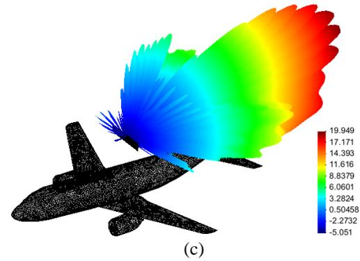
Fig. 13. 2D and 3D gain patterns of the airborne array antenna: (a)  $xoy$  plane, (b)  $xoz$  plane, and (c) 3D pattern.
