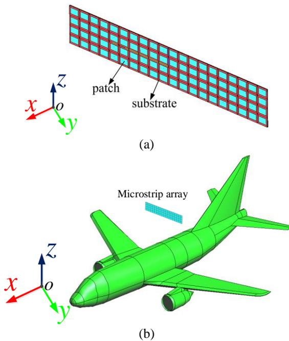
Fig. 12. The airborne array model: (a) the microstrip patch array with  $20 \times 4$  elements, and (b) the airborne microstrip patch array.
