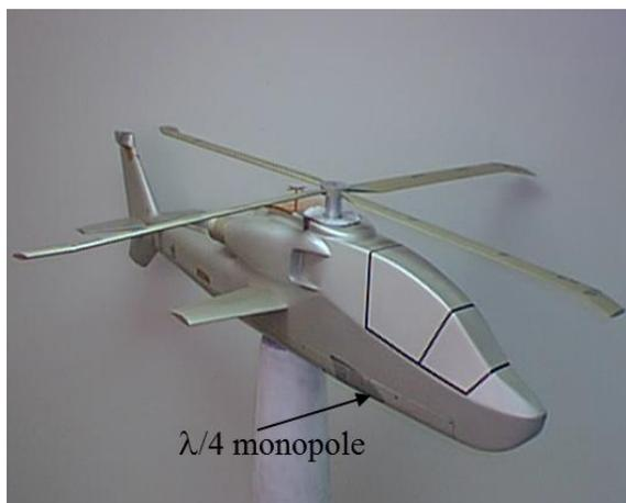
(a) Scale model helicopter (10:1 scale)
