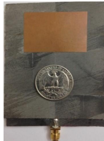
Fig. 6. Top view of the fabricated antenna.
