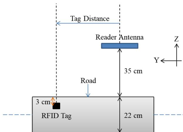
Fig. 1. Side view of the simulation setup. The pavement is infinite in the X and Y directions. The RFID tag antenna and reader antenna are linearly polarized in the X direction.
