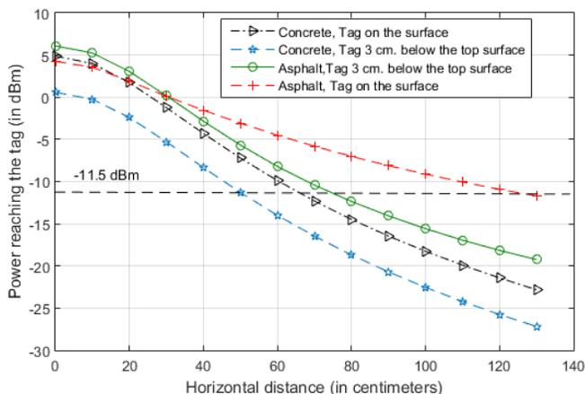
Fig. 2. Power received by the tag antenna as a function of the horizontal distance from the reader antenna for tags on or inside concrete and asphalt pavement. The threshold power of -11.5 dBm is required to activate the RFID chip.
