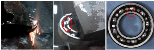
Fig. 7. The damage process using electric discharge machine.
