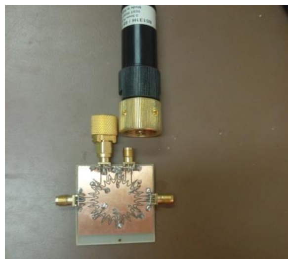
Fig. 3. A photograph of the measured coupler with bond wires and connectors (port 2 is match terminated).
