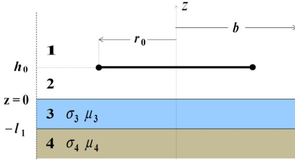
Fig. 2. Rectangular cross-sectional filamentary coil located above a two-layered conductive half-space.
