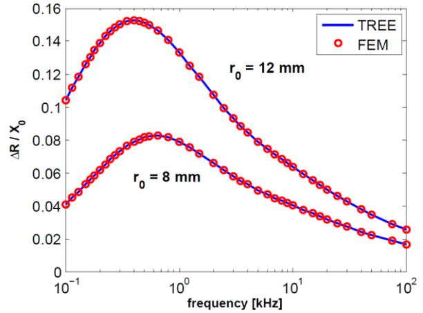
Fig. 4. Real part of the normalized impedance change as a function of frequency for filamentary coil.
