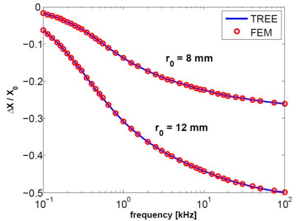
Fig. 5. Imaginary part of the normalized impedance change as a function of frequency for filamentary coil.
