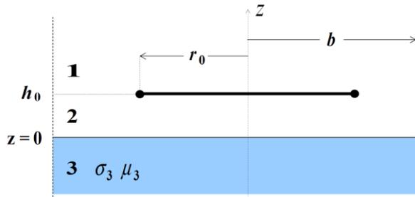
Fig. 3. Rectangular cross-sectional filamentary coil located above a conductive half-space.
