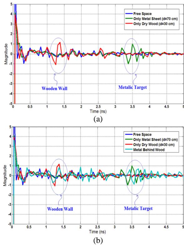
Fig. 7. Measured reflected signal from see through the wall experimental setup: (a) detection of the wooden wall and the metal target separately, and (b) detection metal target behind the wooden wall.
