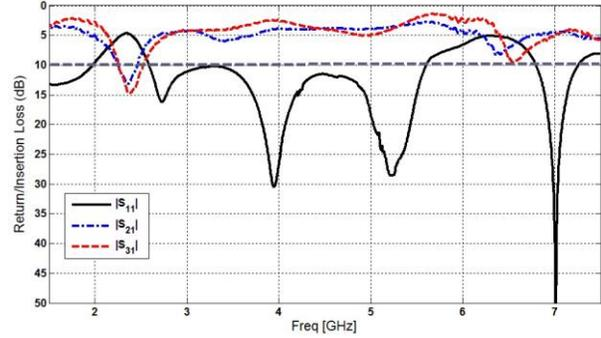
Fig. 4. Measured return and insertion losses for the proposed power combiner.
