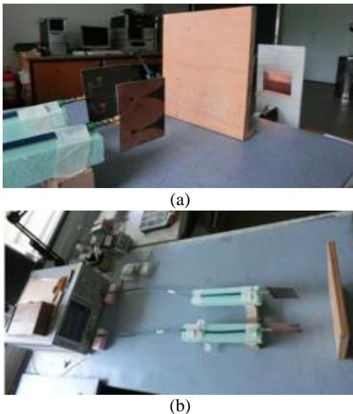
Fig. 6. Experimental setup of the down range resolution measurement using dihedral as radar object: (a) antennas, wooden wall and metal target, and (b) VNA using as a FMCW transceiver.
