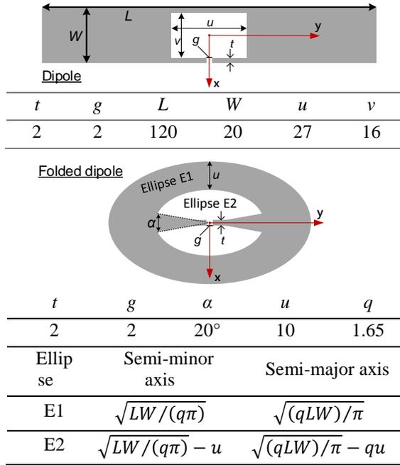
Fig. 1. Structural diagrams of the studied antennas.
