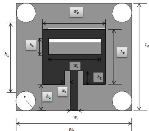
Fig. 2. Front and back view of the proposed dual-band antenna.
