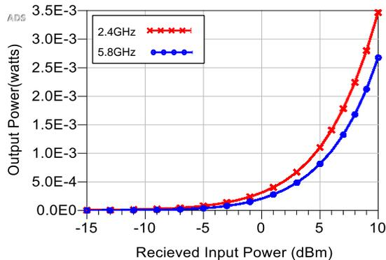
Fig. 6. Output power versus input received power at 2.4 GHz and 5.8 GHz.
