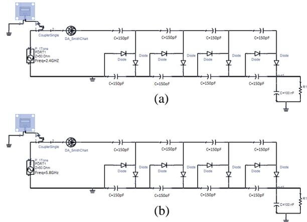
Fig. 4. Schematic diagram of 4-stage RF energy harvesting system for: (a) 2.4 GHz and (b) 5.8 GHz.
