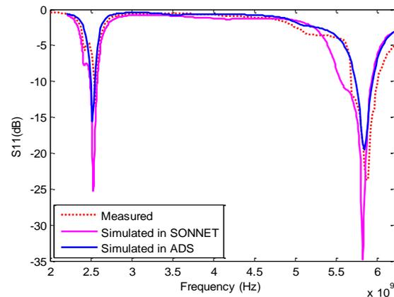
Fig. 5. Input reflection coefficients (S11) of the proposed antenna.
