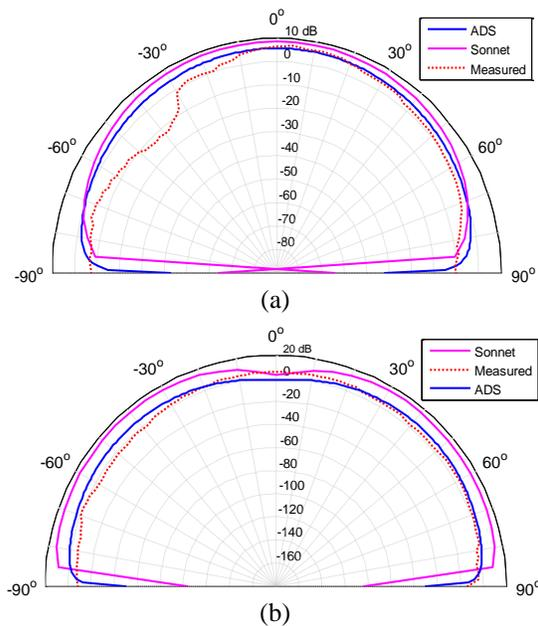
Fig. 7. Directivity of the antenna: (a) at 2.4 GHz and (b) at 5.8 GHz.
