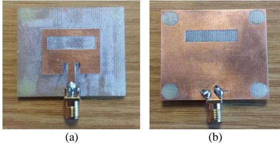
Fig. 3. Prototype of the designed antenna: (a) front view and (b) back view.
