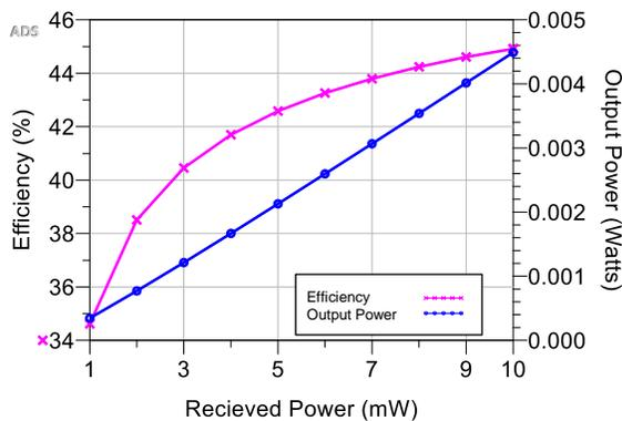
Fig. 9. Effect of incident RF power on efficiency of the proposed system.
