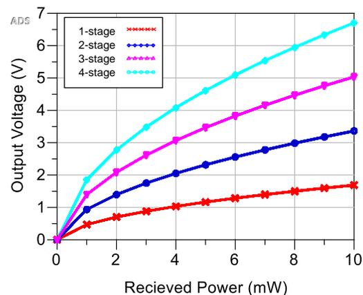
Fig. 8. Effect of number of stages on the output voltage.
