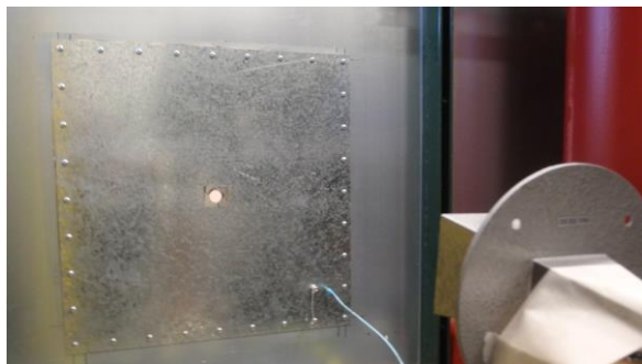
Fig. 8. Transmit antenna position (external to the chamber) for measuring coupling of the electromagnetic wave through the opening, 18 GHz to 40 GHz.
