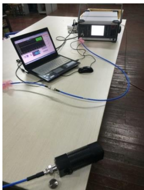
Fig. 4. A measuring system composed of a PIM analyzer, a computer and device under test.
