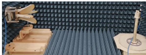
Fig. 7. Experimental setup for measurement of the antenna radiation patterns.
