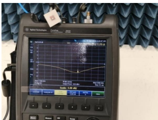
Fig. 5. Experimental measurements of S_{11} for the circularly polarized patch antenna using vector network analyzer of the Agilent Field Fox N9918A.
