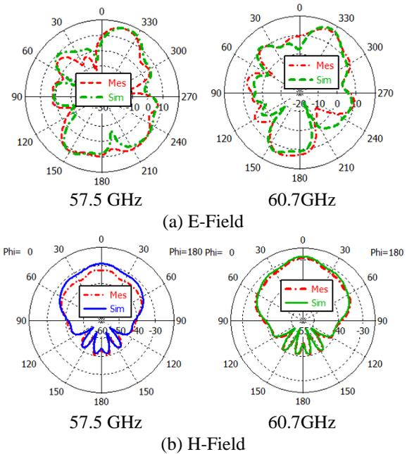
Fig. 6. Farfield patterns at resonant frequencies: (a) E-Field and (b) H-Field.
