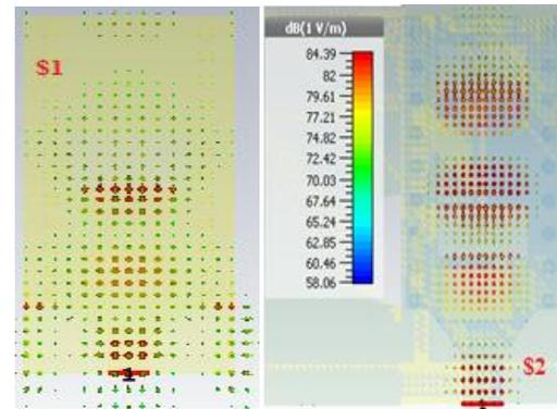
Fig. 8. E-field distribution at 60GHz.
