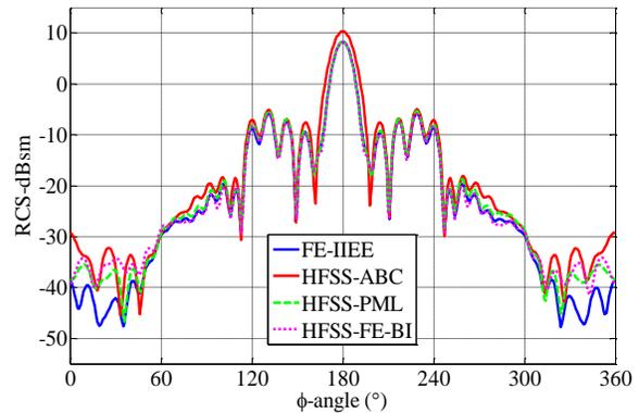
Fig. 7. Bistatic RCS results of the low scattering carrier at 3.0 GHz in the  $xoy$ -plane calculated by the HFSS and the proposed method.
