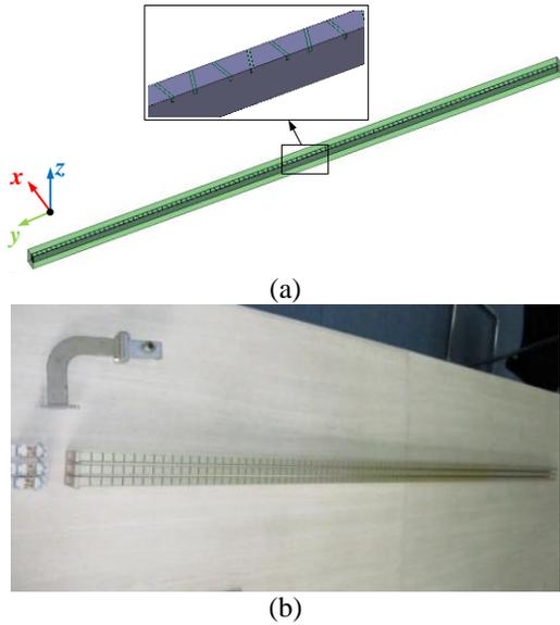
Fig. 8. The waveguide narrow-edge slot antenna model: (a) the simulation model, and (b) the measurement model.
