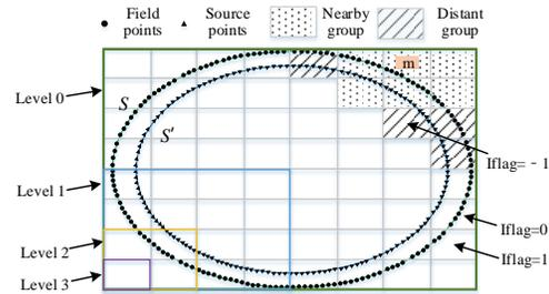
Fig. 2 Configuration for MLFMA based near-field computation.
