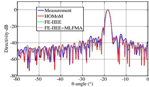
Fig. 9. Normalized radiation pattern of the waveguide narrow-edge slot antenna in the yoz-plane.
