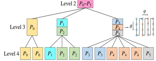
Fig. 4. The parallel strategy of MLFMA for near field computation.
