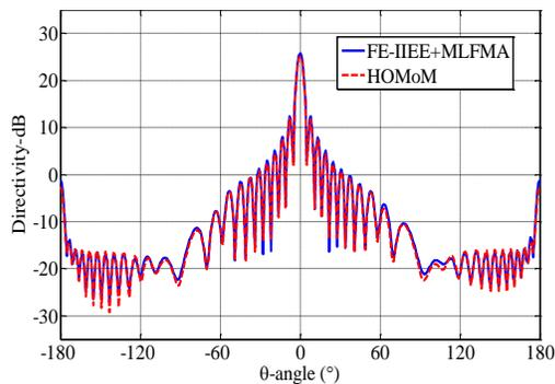
Fig. 11. Radiation pattern of the 100-elements array antenna in the  $xoz$ -plane.
