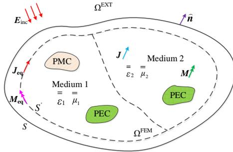
Fig. 1. A typical FE-IIIEE method for general radiation or scattering problems.
