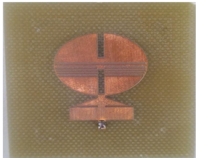
Fig. 4. Top view of the produced antenna.
