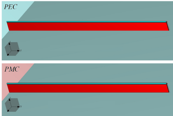
Fig. 7. Transmission line models a towel bar antenna supported by dielectric standoffs, over PEC and PMC planes, in WIPL-D Pro.
