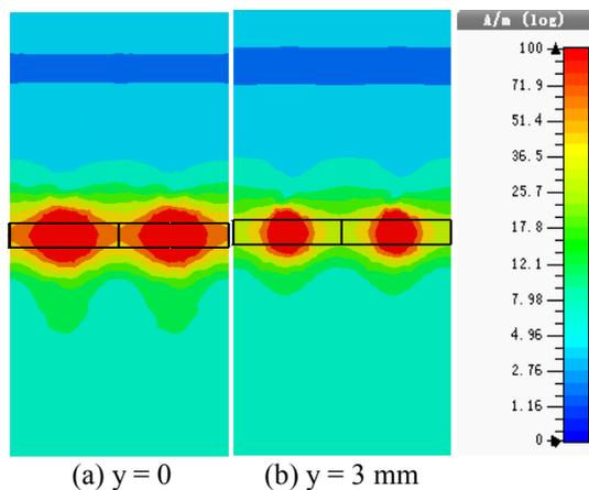
Fig. 8. Cross section of magnetic field distribution in double-layer metal wire structure.
