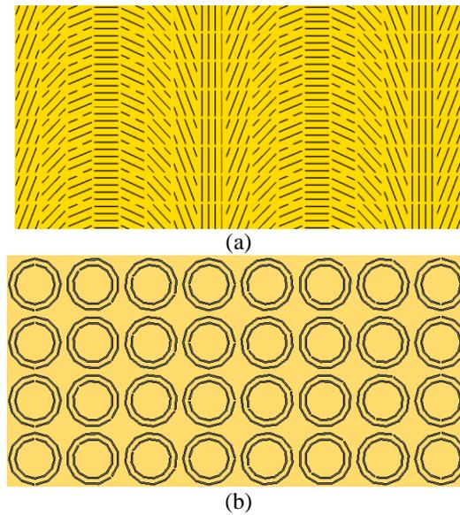
Fig. 9. (a) Metasurface with double-layer metal wire array structure. (b) SRR structure metasurface.
