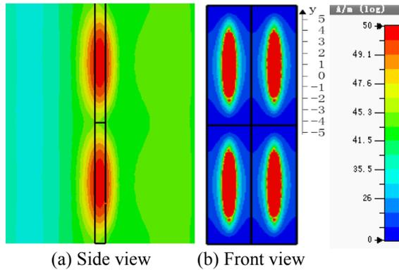
Fig. 7. Simulation of magnetic field distribution in double-layer metal wire structure.
