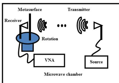
Fig. 11. Measurement setup of the designed metasurface.
