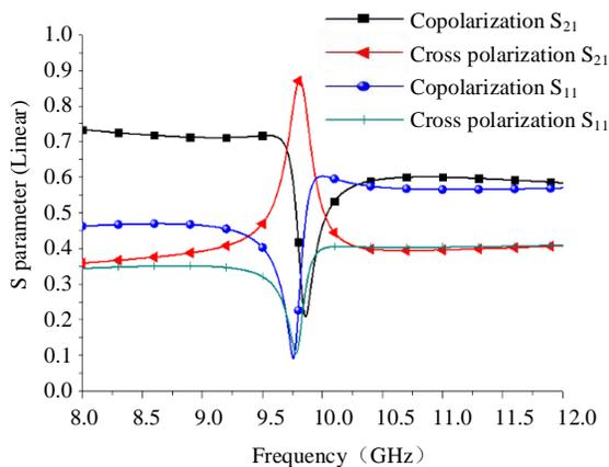
Fig. 4. S parameter simulation results of double-layer metal wire structure.
