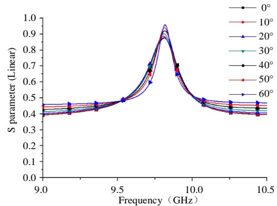
Fig. 5. Oblique incidence cross polarization conversion coefficient of double-layer metal wire structure.
