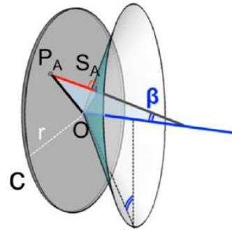
Fig. 2. Plane lens and its equivalent prism.
