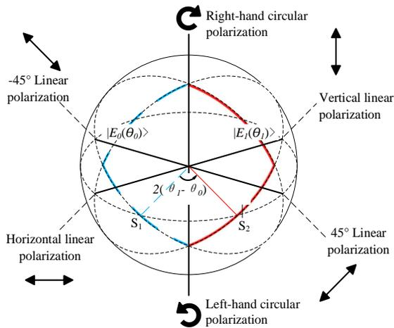
Fig. 1. Polarization representation on Poincare Sphere.
