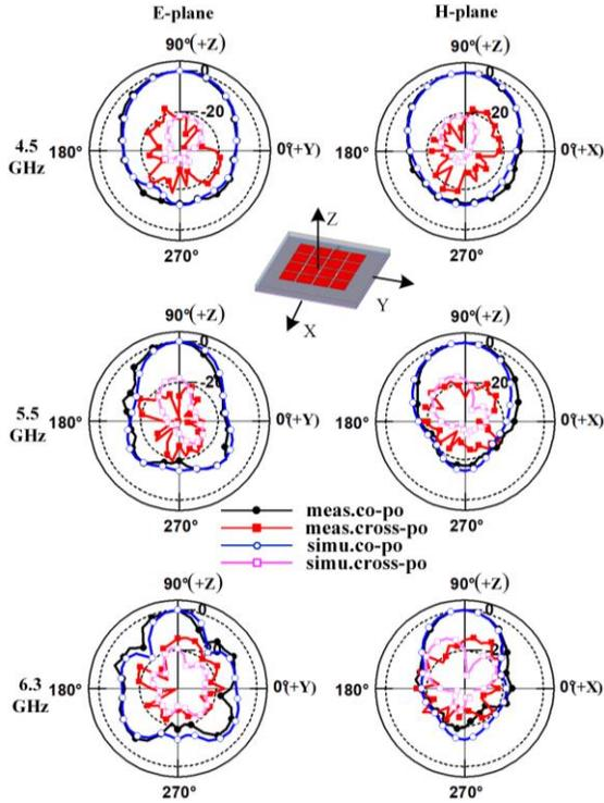
Fig. 8. Simulated and measured normalized radiating patterns at port 2 of the Proposed Ant. at 4.5 GHz, 5.5 GHz and 6.3 GHz.
