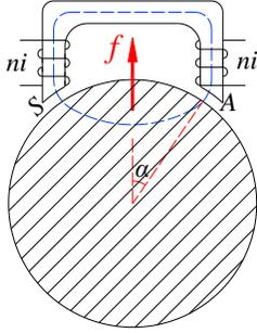
Fig. 1. A couple of magnetic poles and a rotor.
