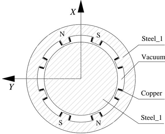
Fig. 3. ANSYS Maxwell model of eight-pole bearing.
