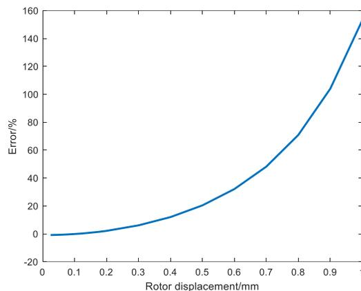
Fig. 9. Effect of rotor displacement on error of  $k_x$ .
