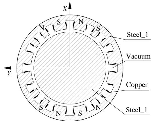
Fig. 7. ANSYS Maxwell model of sixteen-pole bearing.
