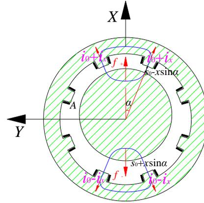
Fig. 2. Force schematic of bearing with eight poles.
