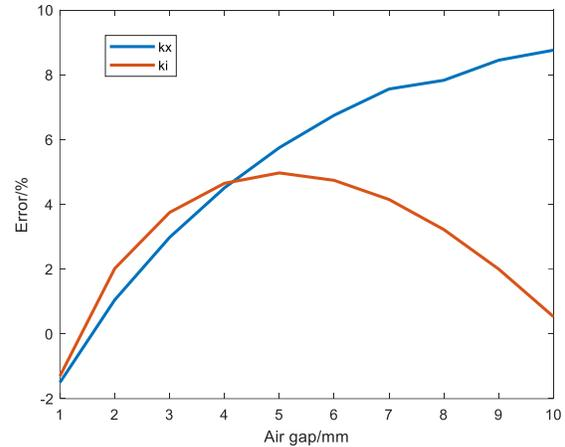
Fig. 8. Effect of air gap on errors of  $k_i$  and  $k_x$ .
