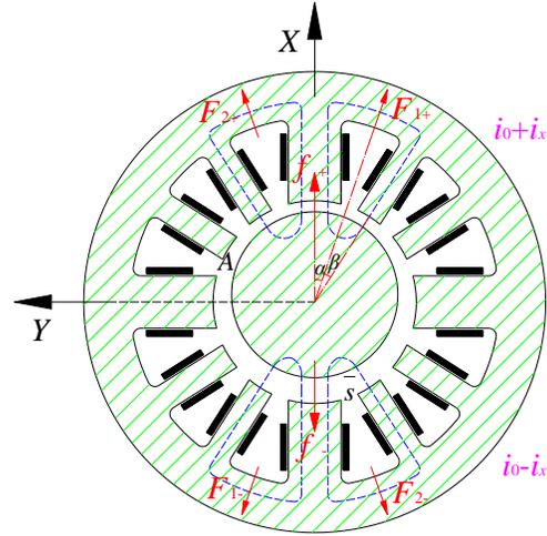
Fig. 4. Force schematic of bearing with twelve poles.
