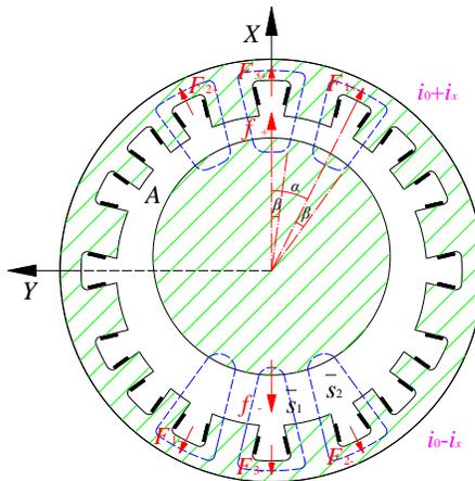
Fig. 6. Force schematic of bearing with sixteen poles.
