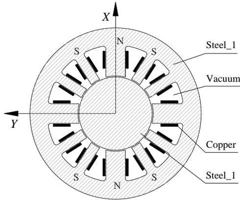
Fig. 5. ANSYS Maxwell model of twelve-pole bearing.
