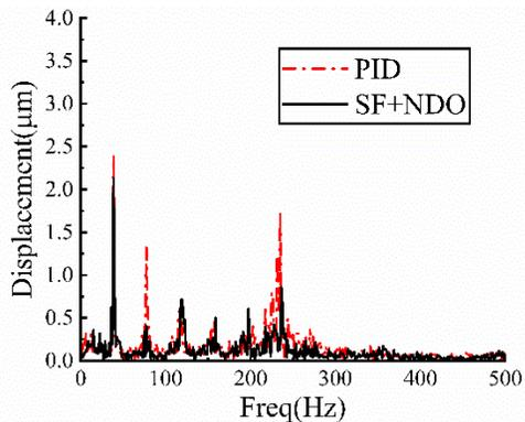
Fig. 11. The spectrum curves of displacement at 2400 rpm.
