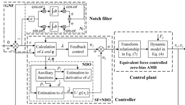
Fig. 3. The whole control system based on SF+NDO+GNF.
