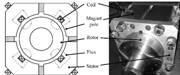
Fig. 5. The structure of the front radial AMB.
