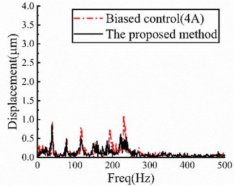
Fig. 13. The spectrum curves of displacement for biased control and the proposed method at 2400 rpm.
