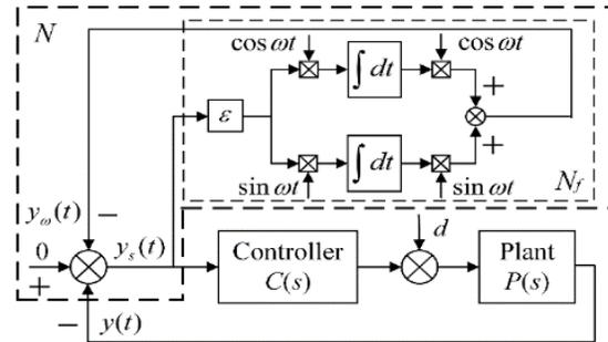
Fig. 2. The principle of the generalized notch filter  $N$ .
