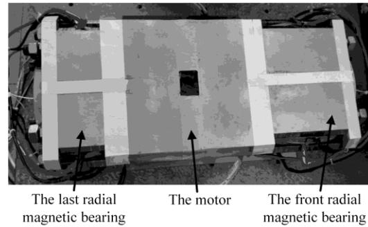
Fig. 4. 5-DOFs magnetically suspended spindle system.
