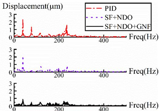
Fig. 12. The spectrum curves of displacement for the three methods at 2400 rpm.
