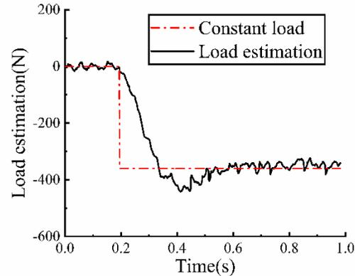
Fig. 9. Load estimation curve under the constant load.
