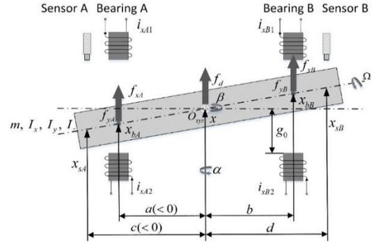
Fig. 1. The diagram of the radial AMBs system.
