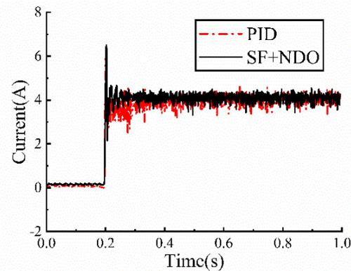
Fig. 7. Current curves during initial lift up.
