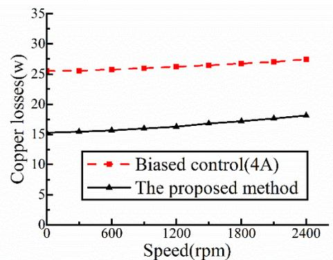
Fig. 14. Copper losses for biased control and the proposed method.
