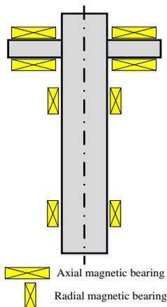
Fig. 2. The AMB structure of atomizer.
