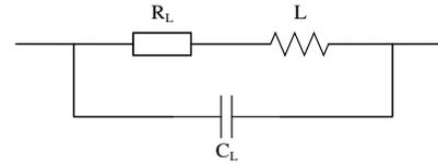
Fig. 7. High frequency equivalent circuit model.
