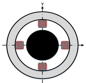
Fig. 3. The structure of differential transformer type displacement sensor used in AMB.
