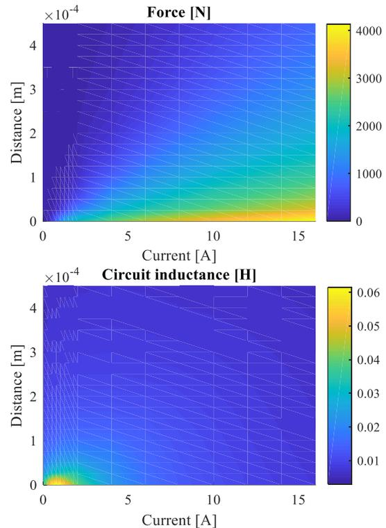
Fig. 3. Look-up tables for electro-mechanical pulling force and circuit inductance.
