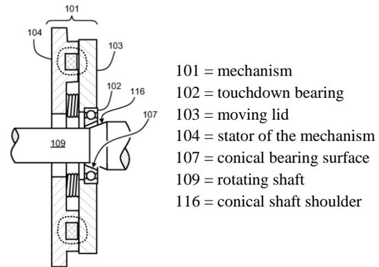
Fig. 1. Schematics and a part list of the studied touchdown bearing mechanism [7].
