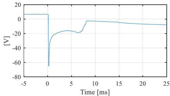
Fig. 6. Voltage profile of the system during a launch.
