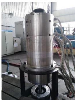
Fig. 1. High speed atomizer.
