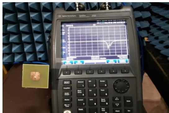
(b) Experimental setup for measuring S_{11}
