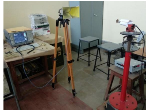
Fig. 5. Experimental setup for the estimation of antenna gain.
