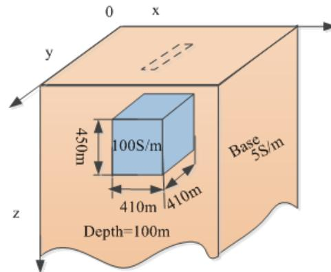
Fig. 4. Anomalous model with single 3D body.
