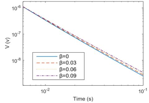
Fig. 1. The induced voltage with different roughness parameters.
