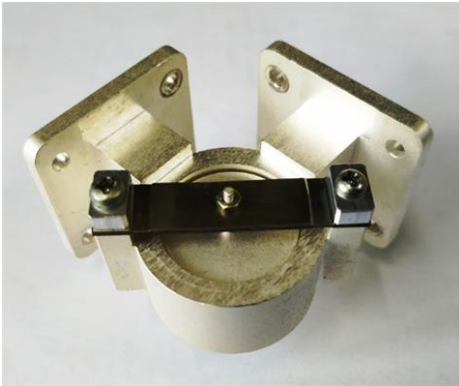
Fig. 9. The photograph of the temperature compensated TE011 mode resonator.
