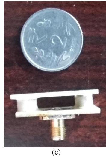
Fig. 2. (a) Metamaterial unit cell, (b) simulated metamaterial superstrate loaded MPA, and (c) fabricated metamaterial superstrate loaded MPA.
