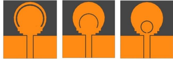
Fig. 2. Placement of resonators, S_1 , S_2 and S_3 in the simulated model.
