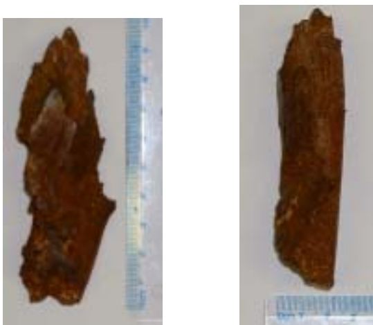
Figure 5. Piece of ordnance scrap on which measurements were performed, with length about 10 cm, width in one transverse direction 3~4 cm and about 2cm in the other.
