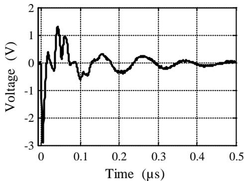
Fig. 8. Voltage measurement inside the stator.
