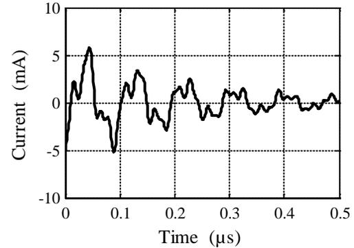
Fig. 12. PD current calculated from the equivalent model.
