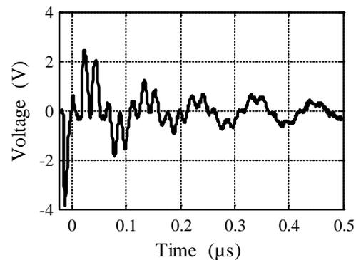
Fig. 6. Voltage pulse measurement on the cable.
