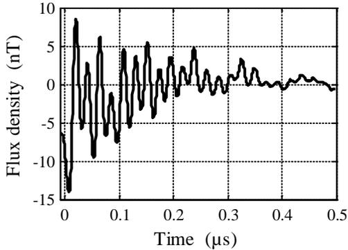
Fig. 7. Flux density due to the partial discharge measured outside the electrical machine.
