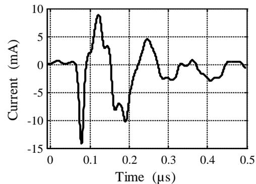
Fig. 10. Partial discharge current in the cable.
