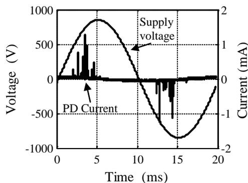
Fig. 5. Partial discharge current (AC-50 Hz).
