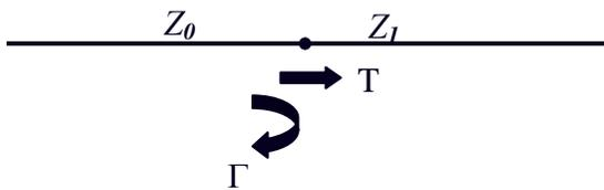
Fig. 2. Illustration of transmission and reflection coefficients.
