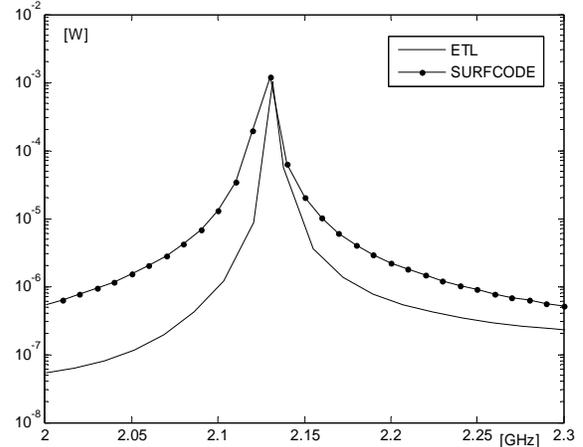
Fig. 5. Absorbed power for ideal dielectric, Case 1.
