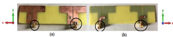
Fig. 9. Fabricated prototype of two element dipole antenna.
