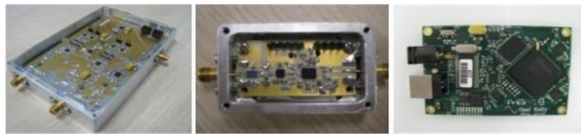
Fig. 4. Photography of the circuit blocks. (Downconverter, RF signal source, and FPGA block).
